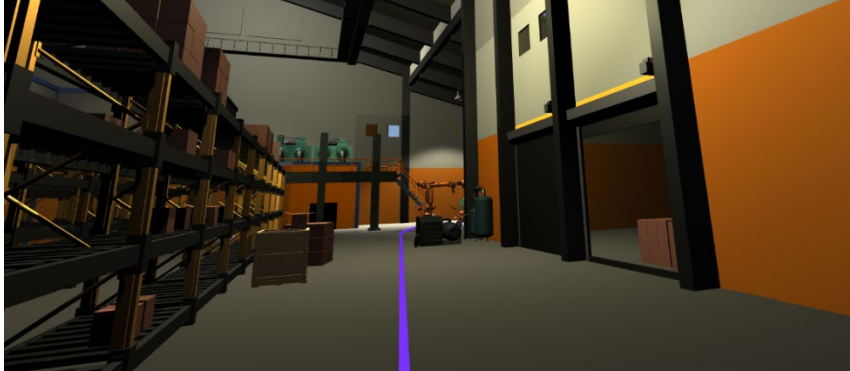
Fig.5. The “follow-the-line” technique uses Unitys NavMesh and LineRenderer function.
